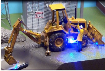
A backhoe contacts an underground line
