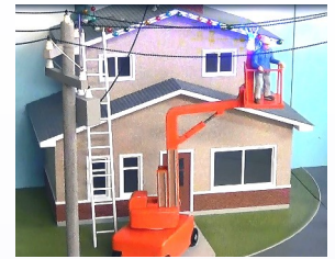
A swing-lift makes contact with an overhead line
