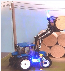
A tractor lifting a hay bale makes contact with an overhead line
